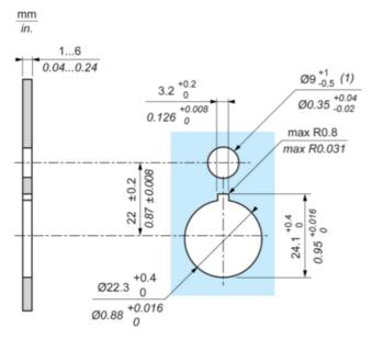
(1) : For IP X9 applications, the max recommendation dimension of hole is  $\emptyset 9 \text{ mm/}\emptyset 0.35$  in.
