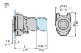
e: clamping thickness: 1 to 6 mm / 0.04 to 0.24 in. (1): Additional row of contacts
