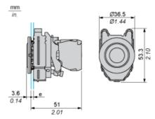
e: clamping thickness: 1 to 6 mm / 0.04 to 0.24 in.
