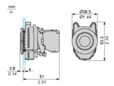
$e: \quad \text{clamping thickness: 1 to 6 mm / 0.04 to 0.24 in.}$
