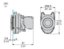
$e: \quad \text{clamping thickness: 1 to 6 mm / 0.04 to 0.24 in.}$
