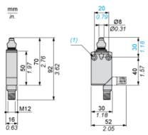
(1) 2 fixing holes  $\varnothing$  4.2 mm, counterbored  $\varnothing$  8 mm by 4 mm deep.
