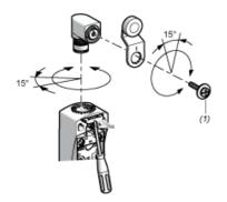
(1) Tightening torque (Min: 1) (Max: 1.5)
