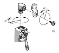
(1) Tightening torque (Min: 1) (Max: 1.5)
